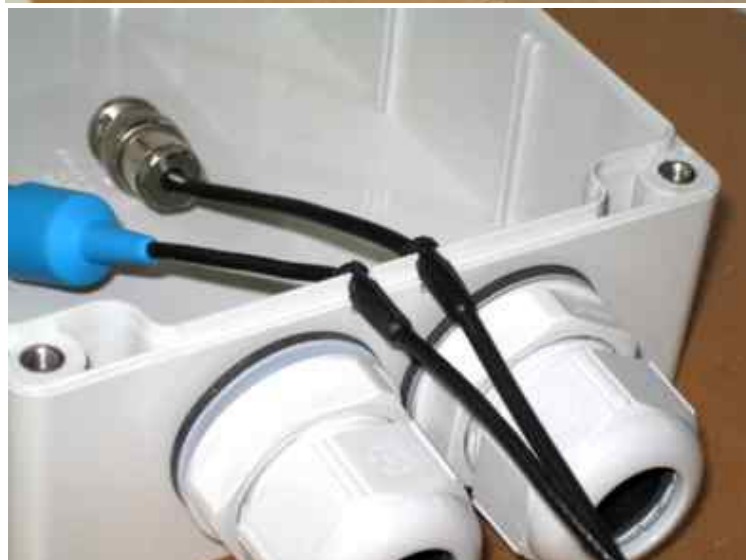
Use the split rubber nipples provide a sealed entry for the pH cables
